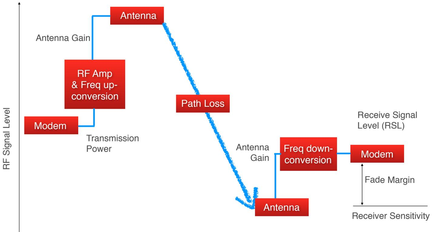
System is operating safely as long as RSL exceeds receiver sensitivity. As path loss varies with transmission environment conditions e.g. temperature, humidity, multi path effect, sizing a point-to-point link means provisioning sufficient Fade Margin to compensate for these variabilities.
